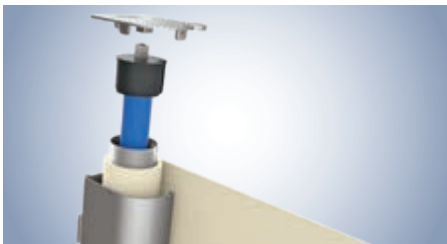
Fabric tensioning via barrel arbor
