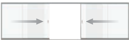
Lockplate version – opens on two sides, closes in the centre
