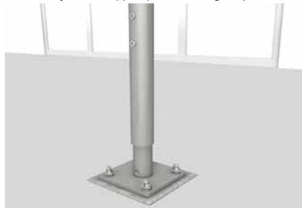
Detail: height adjustment at the base of the front support posts during installation approximately 10 cm
