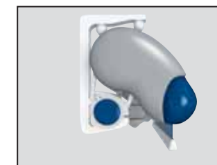
Side view of top-fixed awning with shadeplus (optional) retracted
